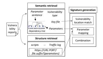
Figure 4: The architecture of signature generation.
